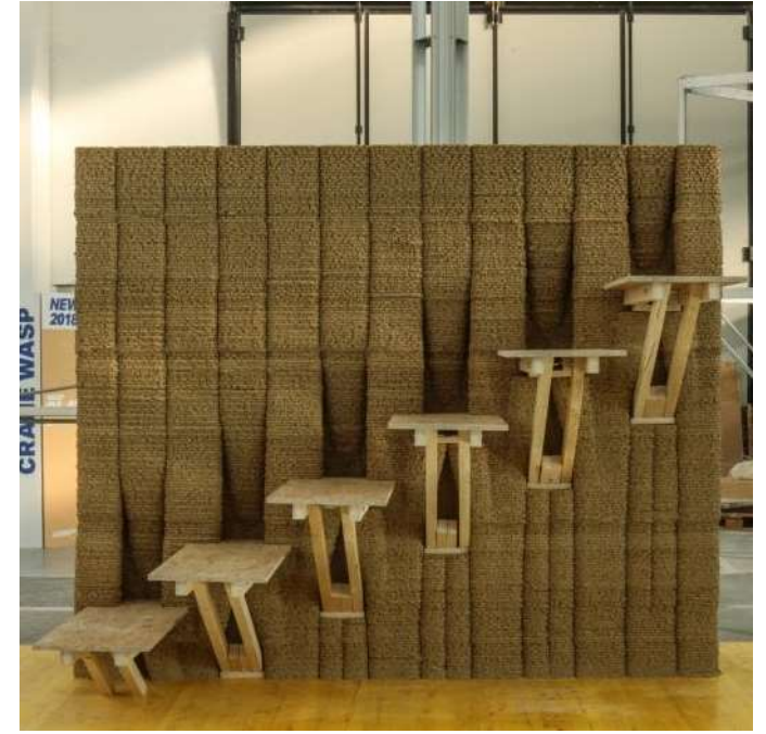
Load bearing earthen wall with timber structure – IAAC & WASP [link]
